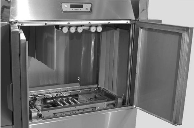
The insulated hinged inspection doors provide easy access in the chamber. Exterior wash pipes and reduced interior baffles reduce clean-up time. The drive allows for a wide separation between the wash and the rinse zone.
