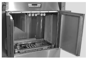
The insulated hinged inspection doors provide easy access in the chamber. Exterior wash pipes and reduced interior baffles reduce clean-up time. The Rapid Return drive allows for a wide separation between the wash and the rinse zone.
