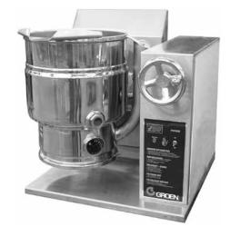
Unit shall be thermostatically controlled to automatically shut off when desired temperature is reached and turn on when product temperature drops below desired setting. Crank till design shall make it possible for one person to easily tilt kettle, even when kettle is filled to capacity. Pouring height allows filling of 4" high pans on the table top.
